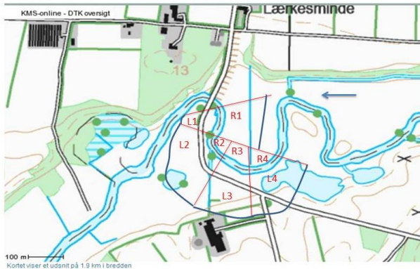
Figure 6: Example of recording sections and boundaries on a topographical map (please avoid the overlapping of adjacent areas at meandering river sites)
